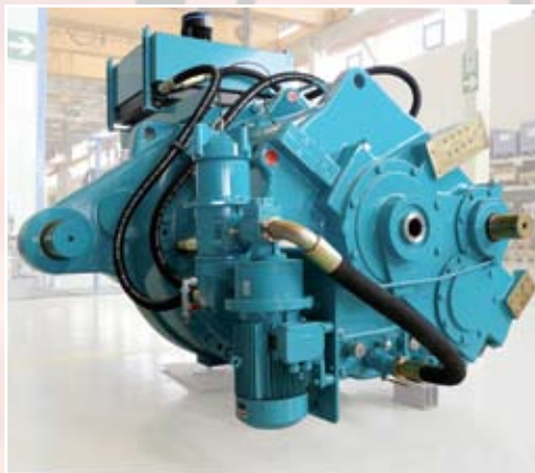
Air Cooled lubrication system with motor / pump filtration system.
